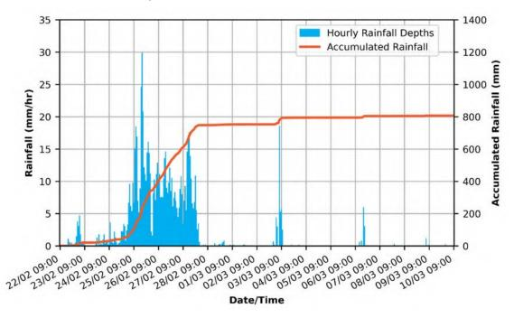
Figure 2-34: Brisbane River from Wivenhoe Dam to Moggill catchment average rainfall in hourly increments and accumulated over the Flood Event for the period 22/02/2022 09:00 to 10/03/2022 09:00
