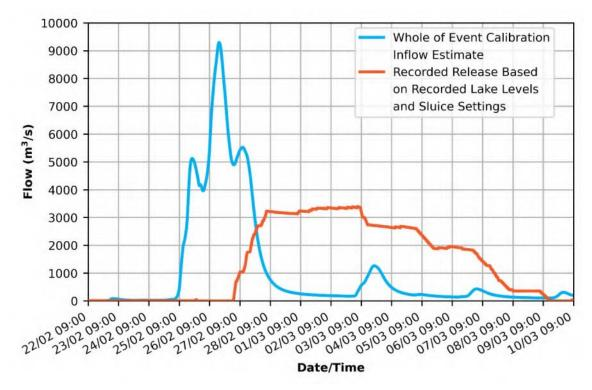
Figure viii: Wivenhoe Dam modelled inflow hydrograph produced by the post-event analysis whole of event calibration (with the benefit of hindsight) excluding Somerset Dam releases and recorded release hydrograph for the period 22/02/2022 09:00 to 10/03/2022 09:00
