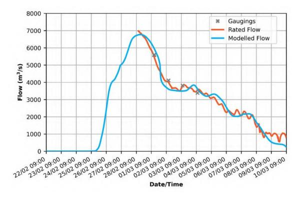
Figure 7-28: Post-event analysis whole of event calibration result (with the benefit of hindsight) at Centenary Bridge compared with rated flow and flow gaugings
