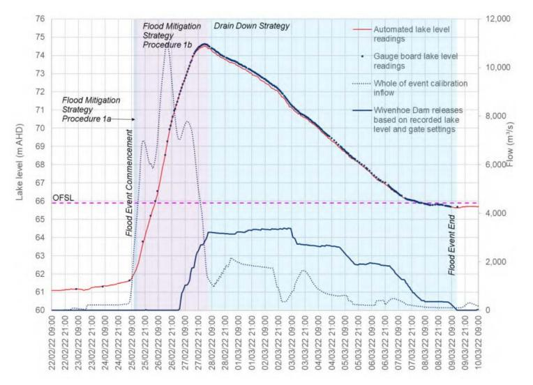
Figure 4-2: Wivenhoe Dam post-event analysis whole of event calibrated inflow, lake level (gauge board and automated readings) and releases (replicated in Figure ii)
