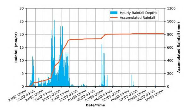
Figure iii: Stanley River to Somerset Dam catchment average rainfall in hourly increments and accumulated over the Flood Event for the period 22/02/2022 09:00 to 10/03/2022 09:00 (replicated in Figure 2-30)
