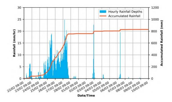
Figure 2-35: Brisbane River downstream of Moggill catchment average rainfall in hourly increments and accumulated over the Flood Event for the period 22/02/2022 09:00 to 10/03/2022 09:00
