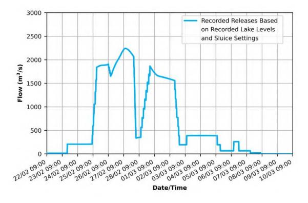
Figure 2-65: Somerset Dam recorded release hydrograph for the period 22/02/2022 09:00 to 10/03/2022 09:00
