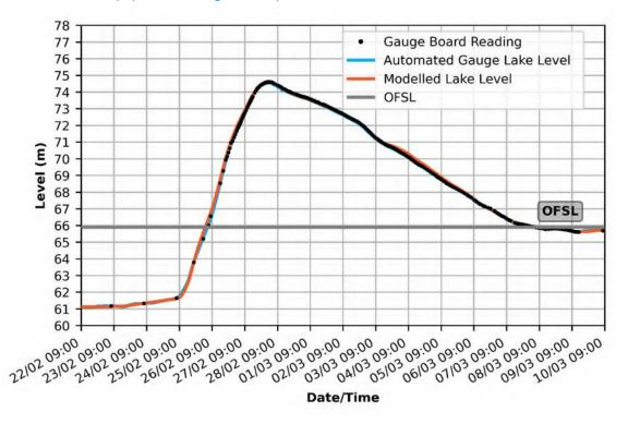
Figure vi: Wivenhoe Dam post-event analysis whole of event modelled lake level compared to automated data and gauge board readings for the period 22/02/2022 09:00 to 10/03/2022 09:00 (replicated in Figure 7-25)
