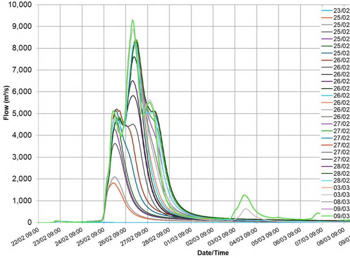
Figure 3-4: Modelled Upper Brisbane River catchment inflow into Wivenhoe Dam (excluding Somerset Dam releases) for each selected key model run
