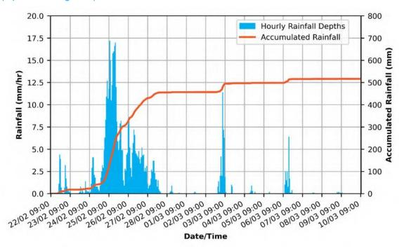
Figure 2-32: Lockyer Creek catchment average rainfall in hourly increments and accumulated over the Flood Event for the period 22/02/2022 09:00 to 10/03/2022 09:00
