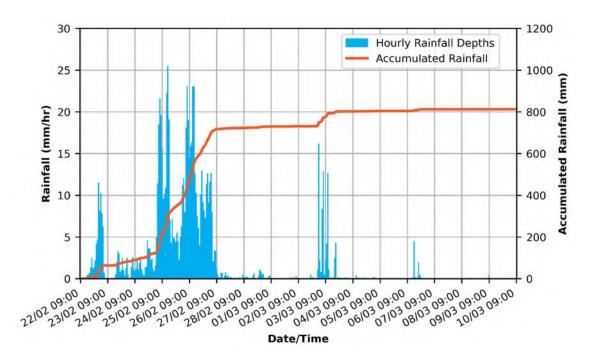
Figure 2-30: Stanley River to Somerset Dam catchment average rainfall in hourly increments and accumulated over the Flood Event for the period 22/02/2022 09:00 to 10/03/2022 09:00 (replicated in Figure iii)
