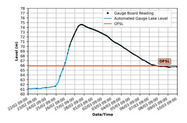
Figure 2-66: Wivenhoe Dam lake level comparing automated water level data and gauge board readings for the period 22/02/2022 09:00 to 10/03/2022 09:00
