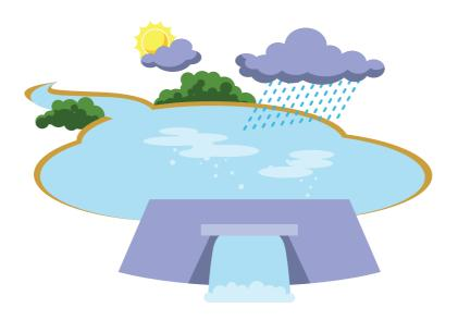
An artificial barrier constructed across a river valley to form a lake for water storage. Any surplus water flows over the dam spillway and down the creek or river.
