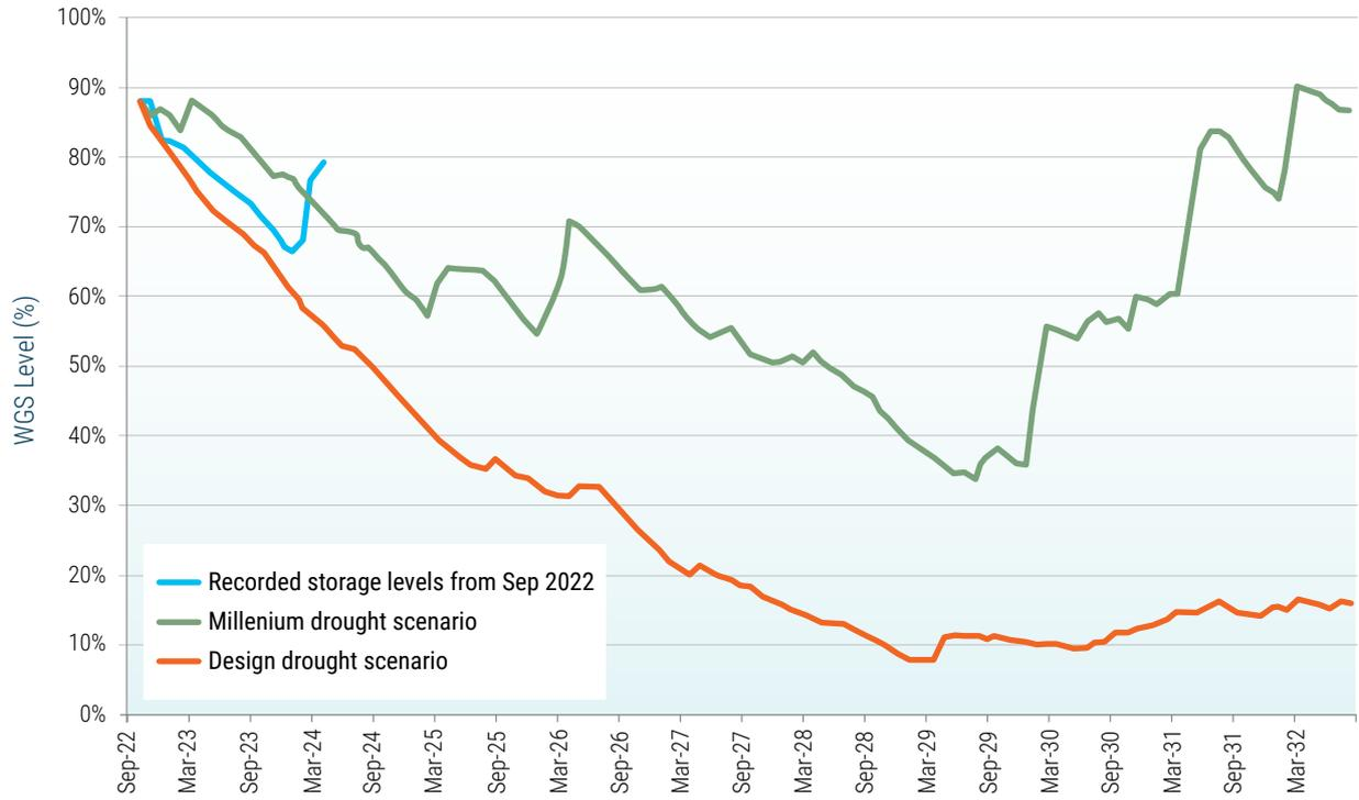
**Figure 4: Design and Millennium Drought inflow draw downs and recorded water grid storage levels from September 2022**
