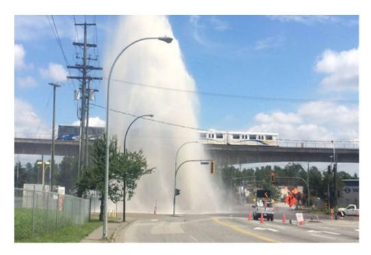
Figure 2-1: Due to the very high pressure at which Trunk water Mains operate; a break has the potential to release dangerous water jets.
