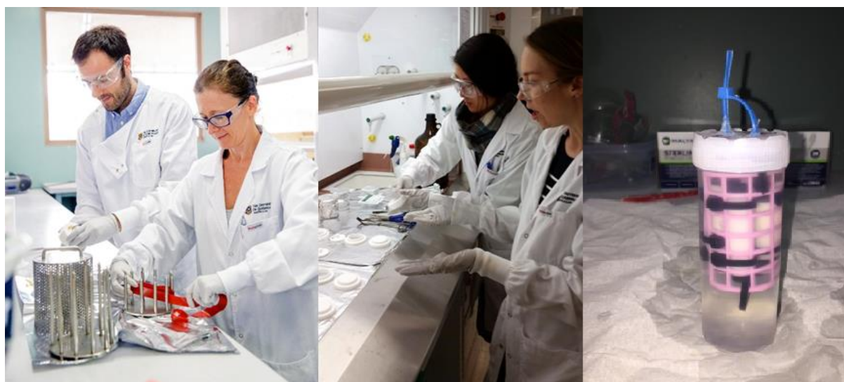
Figure 1. From left to right. Preparation of PDMS passive sampler in stainless steel cage, preparation and assembly of ED passive samplers and deployment setup for a PE passive sampler.
