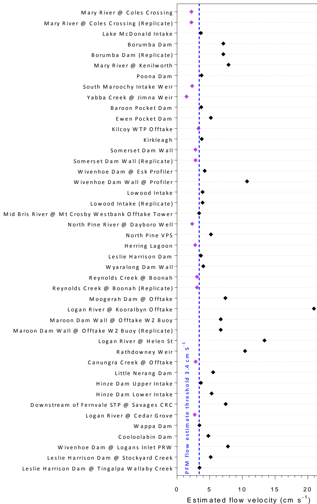
Figure 3. Passive flow monitor (PFM) based average water flow rate estimations at the deployment sites ( n=38 ). A minimum flow velocity of 3.4 \text{ cm s}^{-1} is used to assess flow velocity using Passive Flow Monitors (PFMs). The sites below minimum flow velocity are highlighted in purple.
