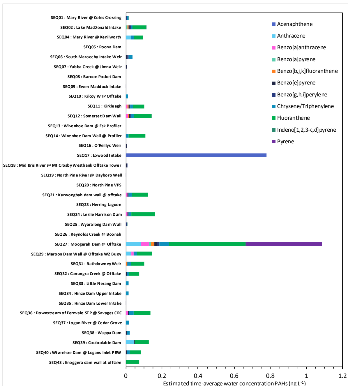
Figure 6. Total estimated water concentrations ( \text{ng L}^{-1} ) of 11 \Sigma PAHs at each site derived from PDMS passive samplers.
