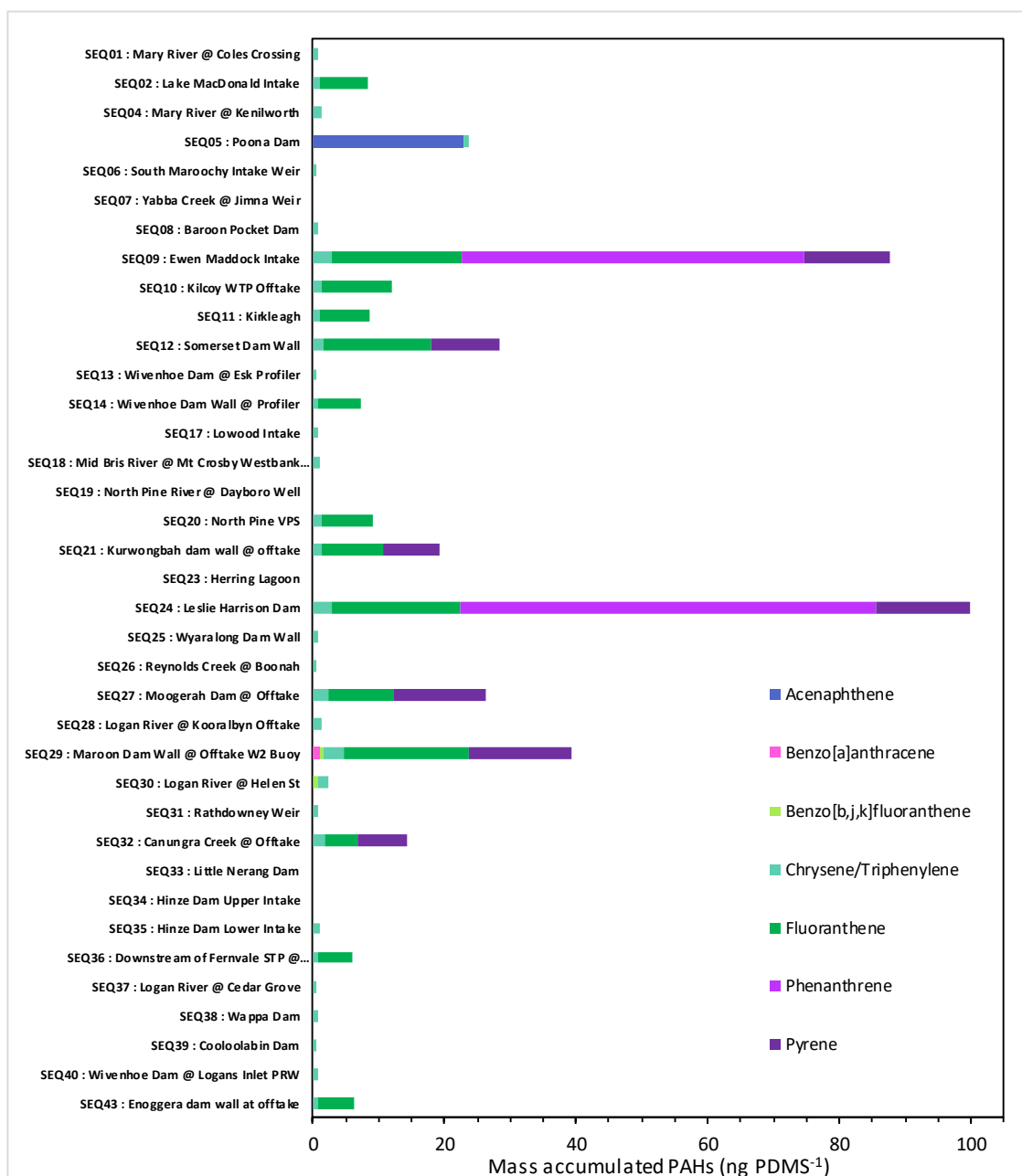
Figure 5. Total mass of 7 \Sigma PAHs ( \text{ng PDMS}^{-1} ) accumulated in PDMS passive samplers at each site.
