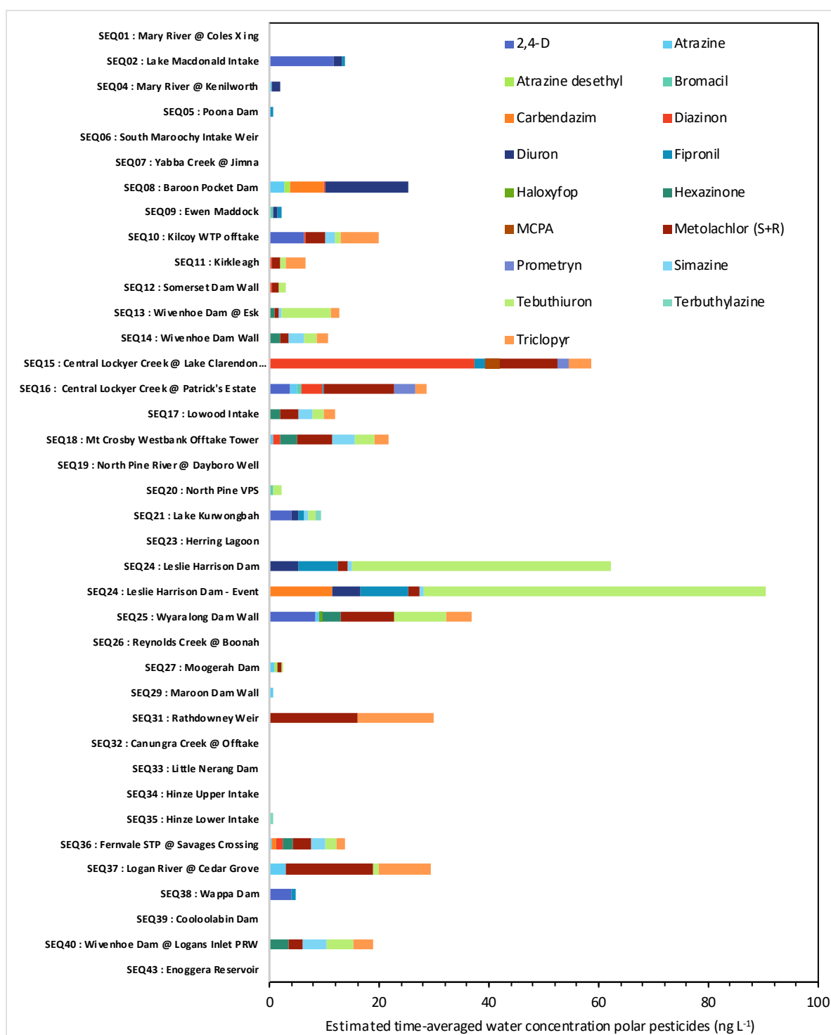
Figure 8. Total estimated water concentrations ( \text{ng L}^{-1} ) of \Sigma Pesticides at each site derived from ED passive samplers.
