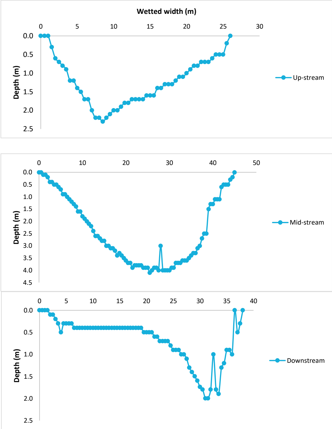
Figure B.3 Site MR4 – channel depth profiles.
