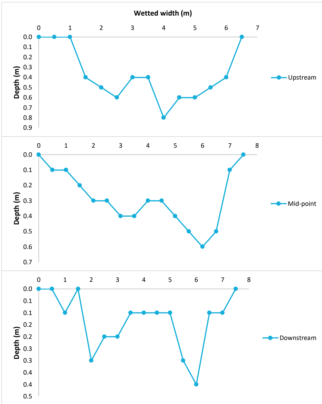
Figure B.4 Site SMC5 – channel depth profiles.
