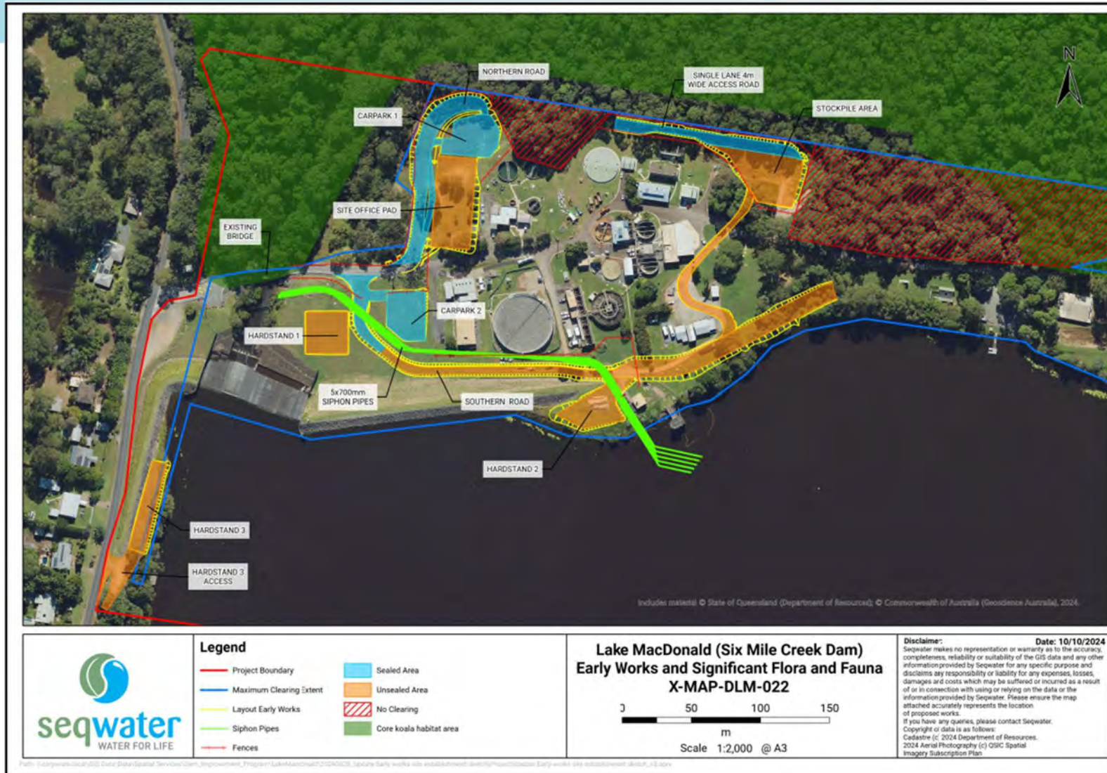
Figure 1: Proposed Early Works Site Establishment Footprint
