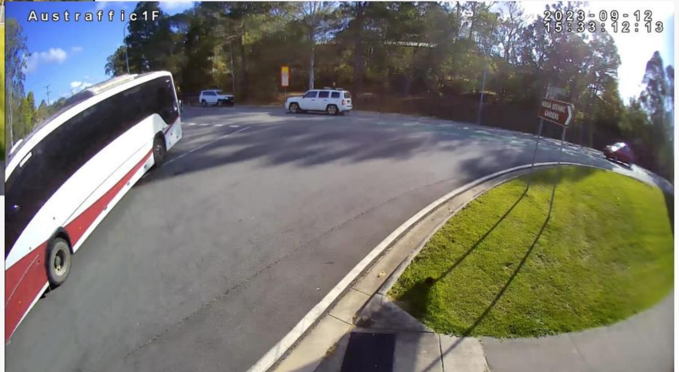
School bus left turn out is over centre line
