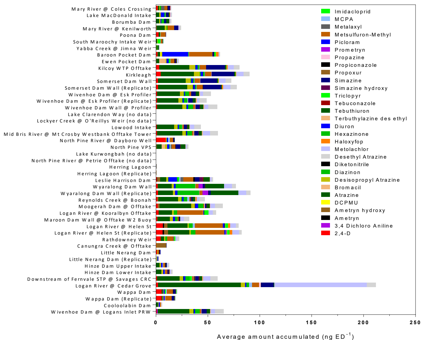
Figure 8. Total amounts (mass) of 30 \Sigma herbicides and insecticides (ng ED -1 ) accumulated in ED passive samplers at each site.
