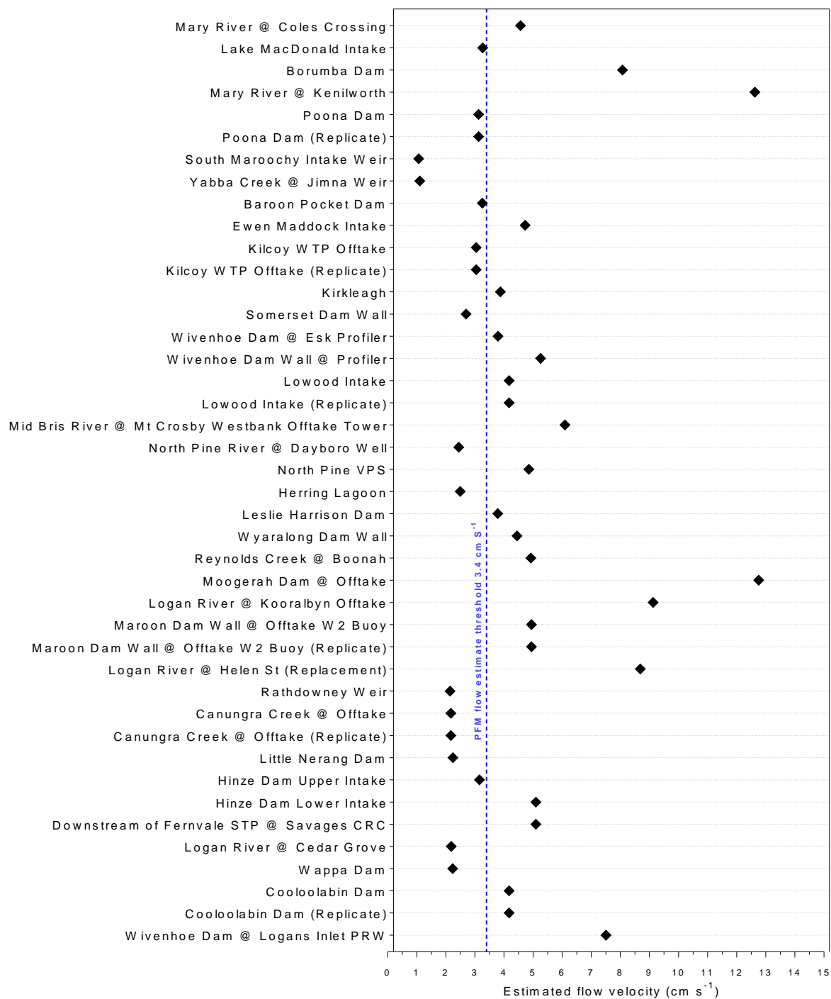
Figure 3. Passive flow monitor (PFM) based water flow rate estimations at the deployment sites ( n=36 ). A minimum flow velocity of 3.4 \text{ cm s}^{-1} is used to assess flow velocity using Passive Flow Monitors (PFMs).
