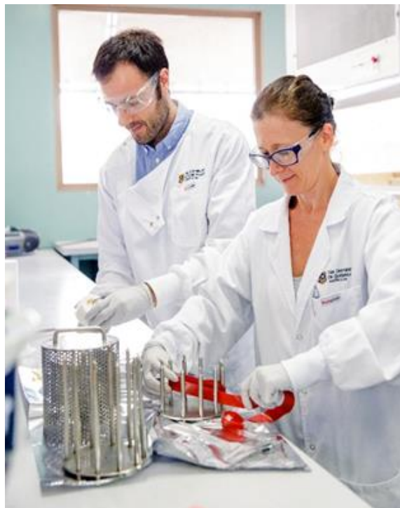
Figure 1. Preparation of a PDMS passive sampler in a stainless steel cage.
