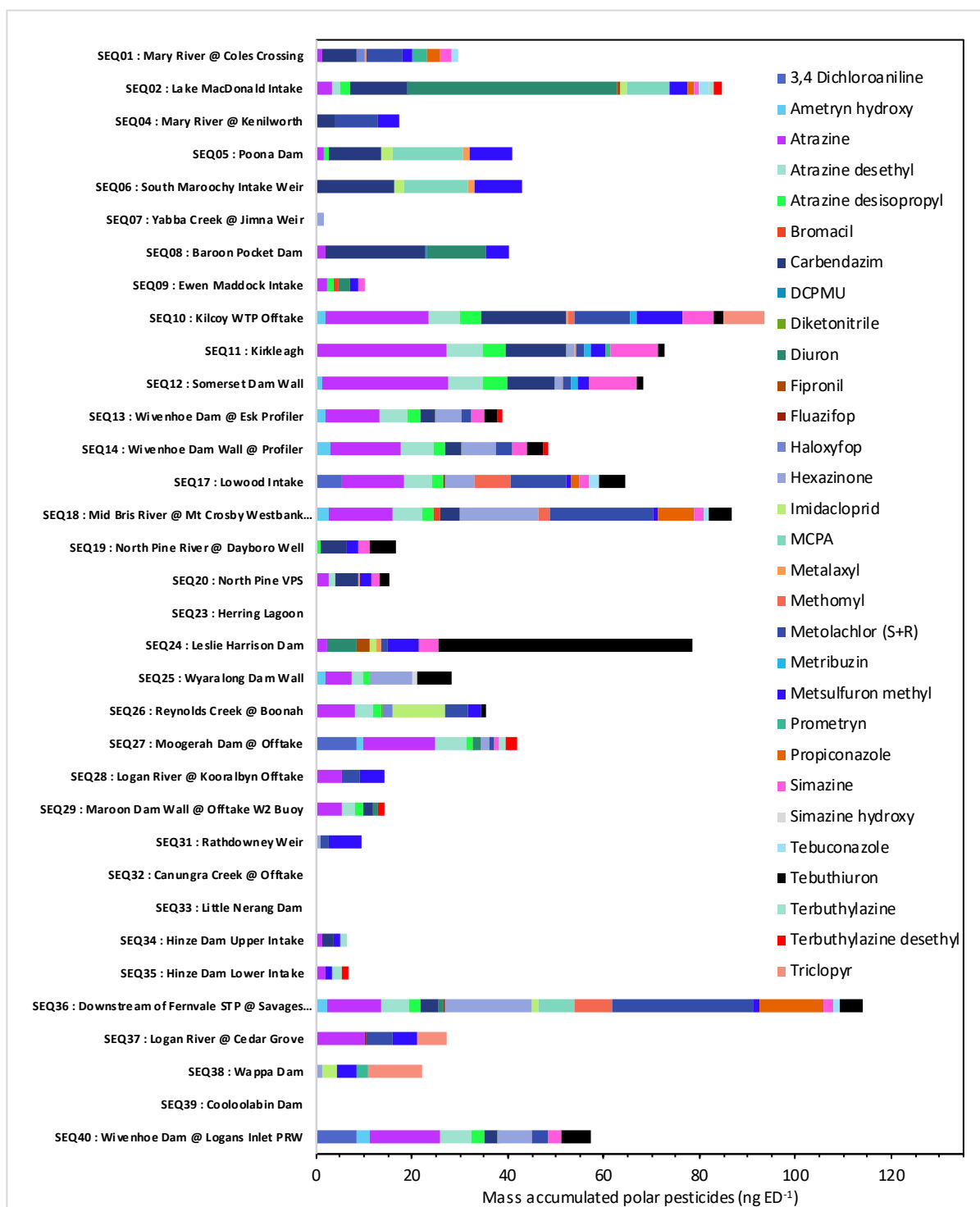
Figure 7. Total mass of 30 polar pesticides (ng ED -1 ) accumulated in ED passive samplers at each site.
