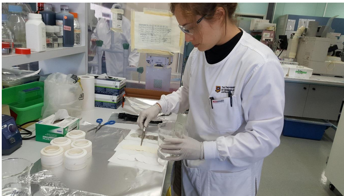
Figure 1 Preparation of Empore Disk (ED) passive samplers for deployment
